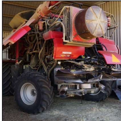
Figure 4: The Harrington Seed Destructor
